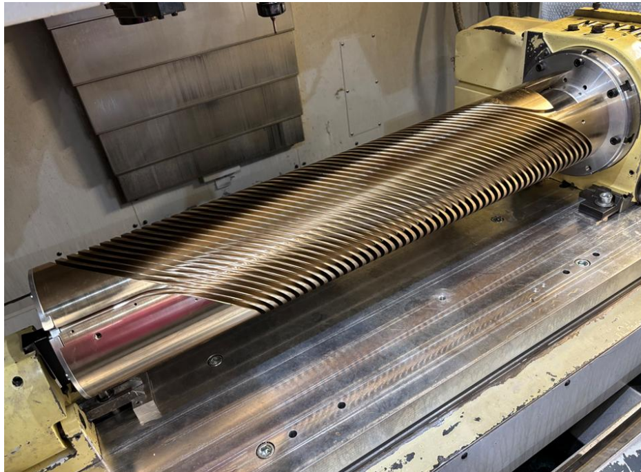
Figure 4. Manufacturing of the outer former.
